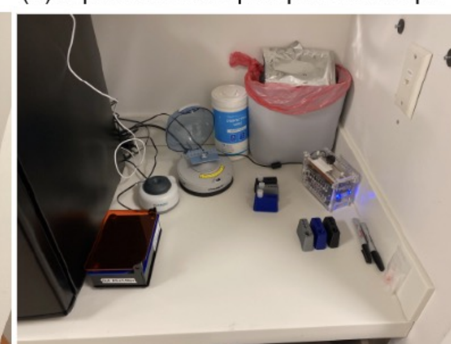
Figure 1. Feasibility of point-of-care RT-PCR COVID-19 test at a pediatric clinic. (A) Kit components (B) Low-cost equipment required to operate our assay including minivortex, minicentrifuge, miniPCR thermal cycler, a mobile phone, and tube racks. (C) and (D) images of the set-up areas to conduct this study in the clinic. (E) Data tracking system via barcodes. HCWs take picture of the barcodes on the tubes before taking images of the tubes to enable accurate data tracking.
